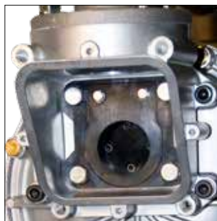
Only 4 bolts to access flap valves
