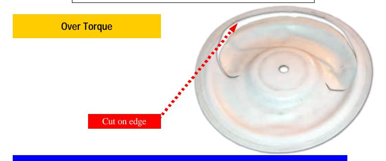
This diaphragm will have a *pronounced cut around its outside edge*. This is caused by the chambers of the pump cutting into the diaphragms due to over tightening (usually metal only). This situation can be avoided by paying close attention to the torque values in the manuals.
