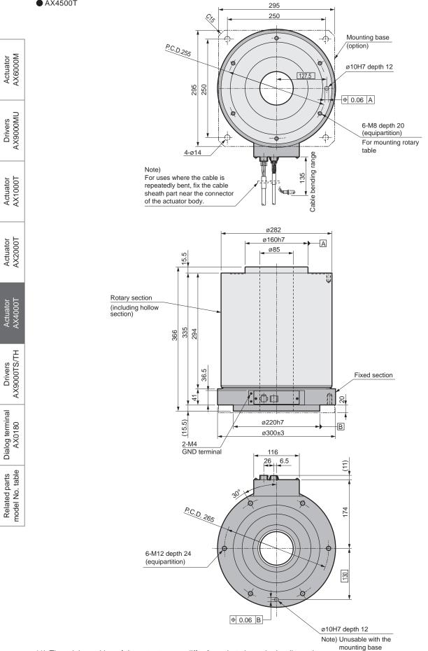
\*1) The origin position of the actuator may differ from that shown in the dimensions. The origin offset function allows you to set a desired origin position.
