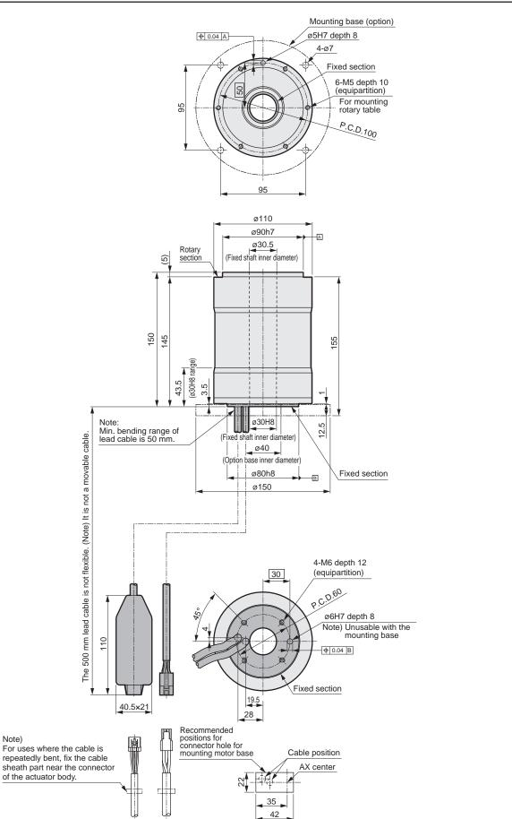
\*1) The origin position of the actuator may differ from that shown in the dimensions. The origin offset function allows you to set a desired origin position.
