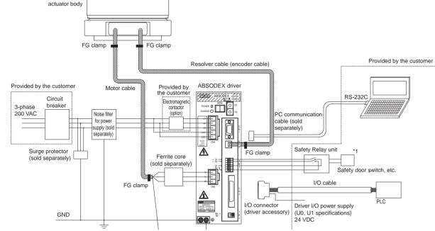
To comply with the CE marking, the parts shown below or overcurrent/short circuit protection Component is required. In addition, the driver must be installed within the switchboard. For details on the selection, installation and wiring methods of these components, refer to the instruction manual or technical data (ABSODEX AX series TS/TH type technical data).
