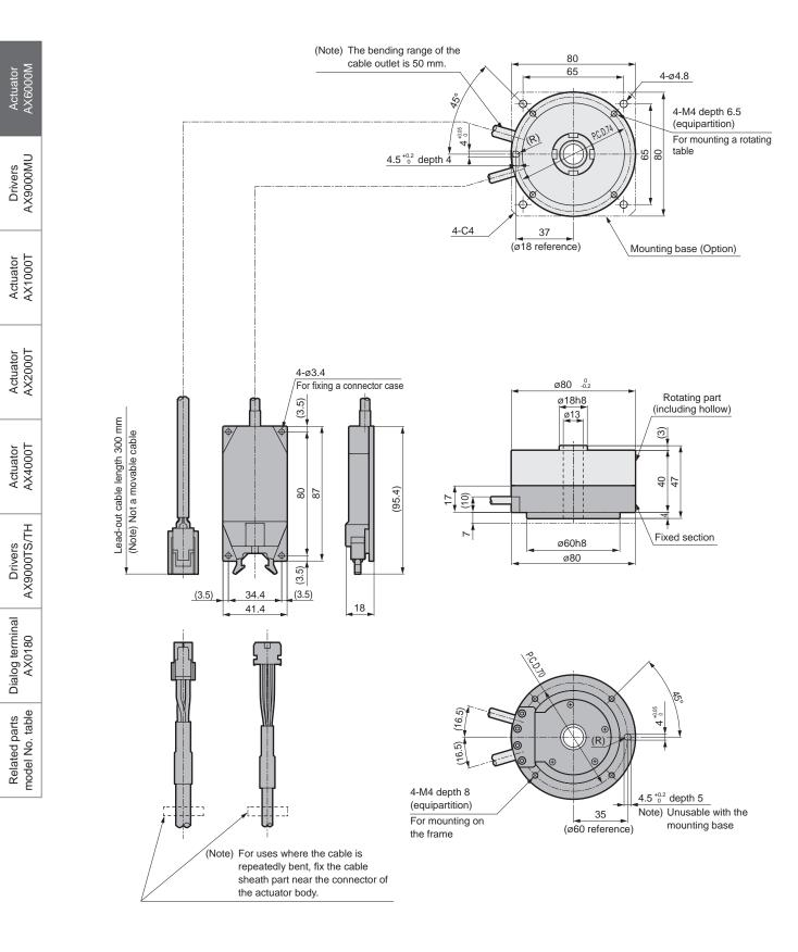
\*1) The origin position of the actuator may differ from that shown in the dimensions. The origin offset function allows you to set a desired origin position.
