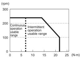
\* Fig. This graph shows the characteristics for 3-phase 200 VAC.
