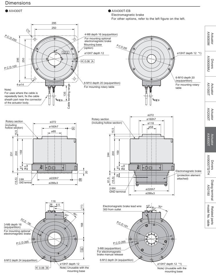
\*1) The origin position of the actuator may differ from that shown in the dimensions. The origin offset function allows you to set a desired origin position. The position of the positioning pin hole is the same as that of AX4300T when an electromagnetic brake is mounted.
