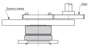
[Fig. 5] Dummy inertia installation example 3
