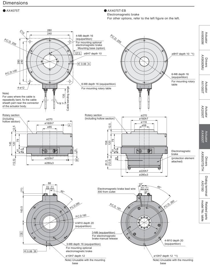
\*1) The origin position of the actuator may differ from that shown in the dimensions. The origin offset function allows you to set a desired origin position. The position of the positioning pin hole is the same as that of AX4045T when an electromagnetic brake is mounted.
