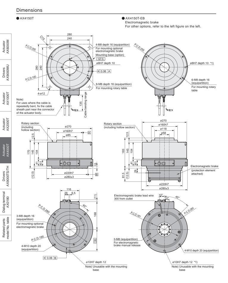
\*1) The origin position of the actuator may differ from that shown in the dimensions. The origin offset function allows you to set a desired origin position. The position of the positioning pin hole is the same as that of AX4150T when an electromagnetic brake is mounted.
