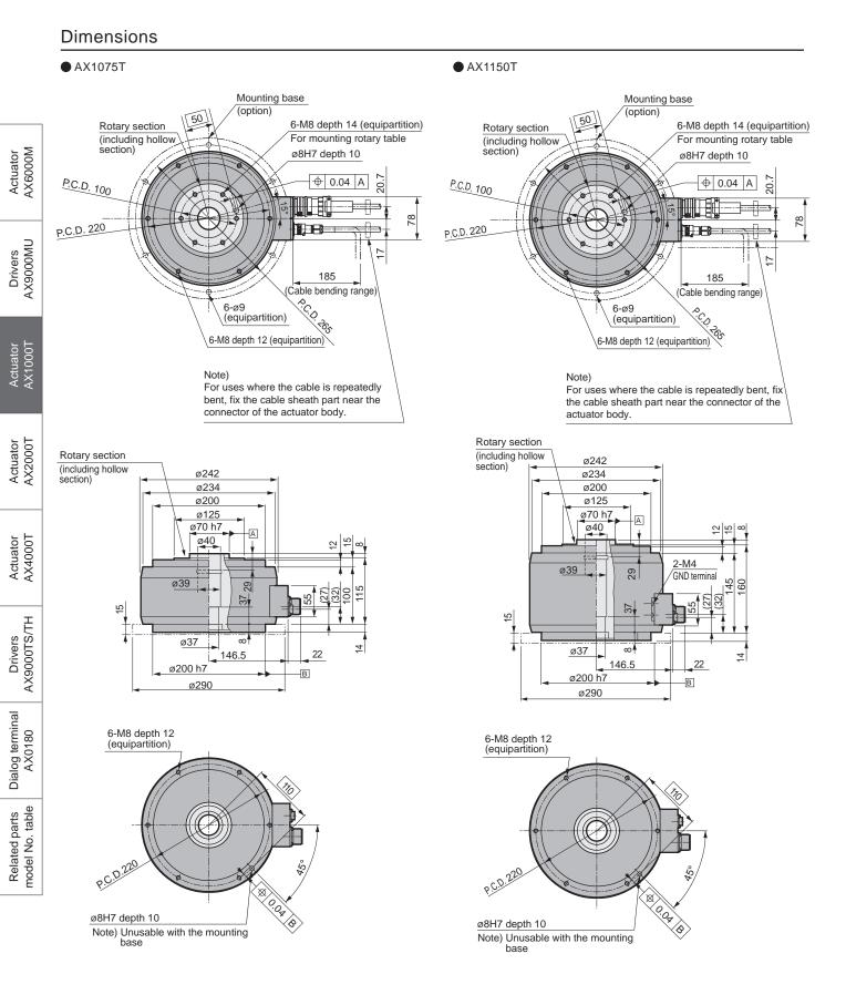
\*1) The origin position of the actuator may differ from that shown in the dimensions.
