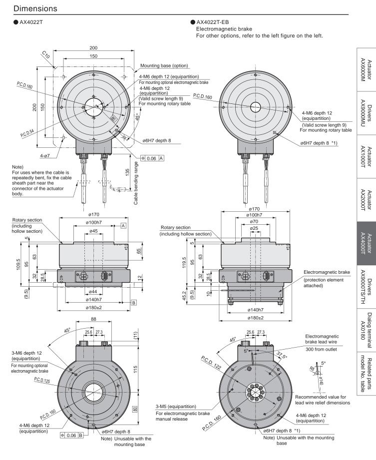
\*1) The origin position of the actuator may differ from that shown in the dimensions. The origin offset function allows you to set a desired origin position. The position of the positioning pin hole is the same as that of AX4022T when an electromagnetic brake is mounted.
