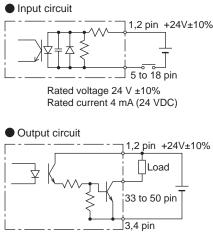
Rated voltage 24 V ±10% Rated current 30 mA (MAX) CN3 Output signal
